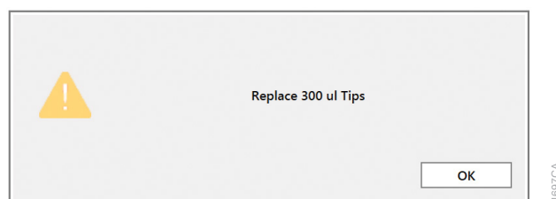
Figure 25. Insufficient tips on the system to complete a method. In the event that all tips of a given tip type are consumed during a run, the instrument will pause and unlock the door. Open the door, load more tips of the indicated type on the tip and plate carrier, close the door and press OK to resume processing.
