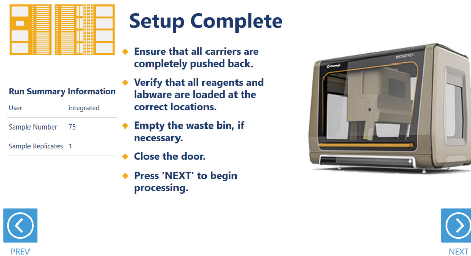
Figure 23. Final instrument setup screen. This screen presents a list of items that should be checked before starting automated processing. It also provides a final chance to return to any of the previous instrument setup screens before automated processing begins. To start processing, close the instrument door and press the Next button.
