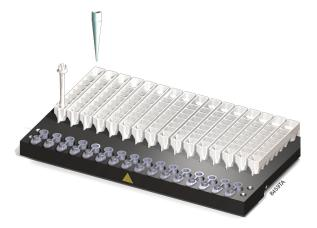
8. Place 0.5ml Elution Tubes in the front of the Maxwell® 16 LEV Cartridge Rack. Add 50μl of Nuclease-Free Water to the bottom of each Elution Tube.
