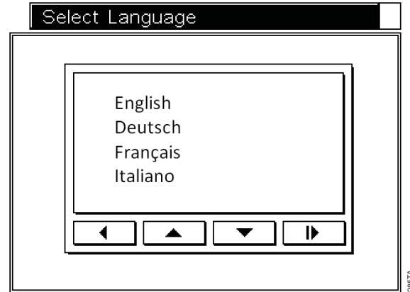
Figure 11. The Select Language screen. Once you have selected a language, press the Run/Stop button.
