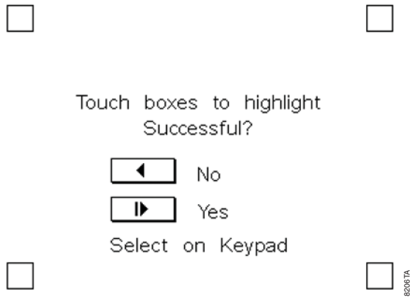
Figure 13. Confirmation screen for the Touch screen. Touch all four boxes, if all change color, press the Run/Stop button on the instrument keypad. If they do not all change color, press the back arrow button and repeat the calibration and confirmation.
