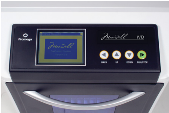
Figure 3. The touch screen and the keypad for use in navigating through the various screen displays for the Maxwell® 16 IVD Instrument. The same button selections are available on the keypad and the screen. Both sets of buttons can be used to navigate within and between screens. The Back and Run/Stop buttons allow navigation between screens. The Up and Down buttons are for navigation within a screen.
